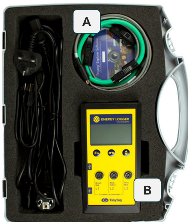
Figure 6-2. Tinytag TGE-0001 Energy Data Logger
