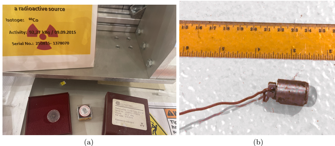
Figure 4.1: Photograph of (a) calibration sources ( ^{22}\text{Na} , ^{137}\text{Cs} , ^{60}\text{Co} ) and (b) PuBeNi source
