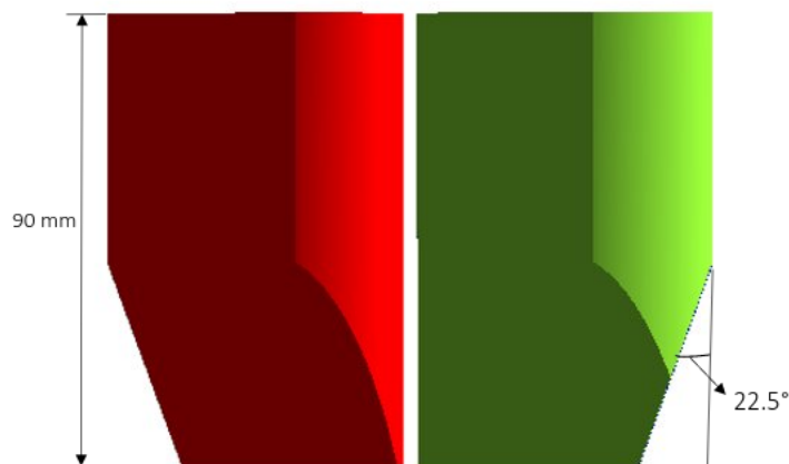
Figure 5.3: The side view of the ELIADe HPGe clover reveals its configuration. The HPGe will be tapered on the outer faces, and in cones on the corners, on an angle of 22.5^\circ to a depth of 36.2 mm. (GEANT4 view)
