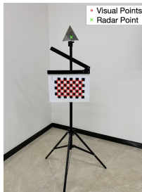
Fig. 2. Calibration target for microphone, camera and radar
