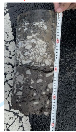
Core Sample of Debonding (3)
