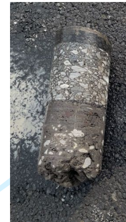
Core Sample of Loosening (3)
