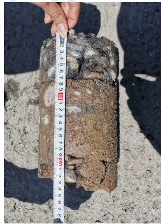
Core Sample of Loosening (2)
