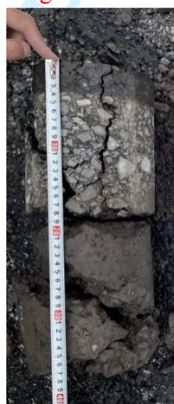
Core Sample of Debonding (2)
