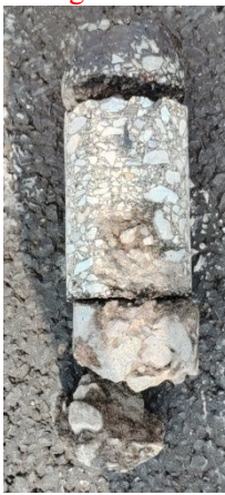
Core Sample of Debonding (1)
