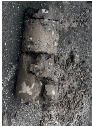
Core Sample of Loosening (1)
