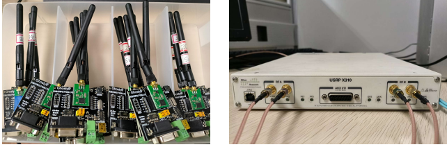
(a) Photo of the 18 ZigBee devices. (b) Photo of the USRP receiver.
