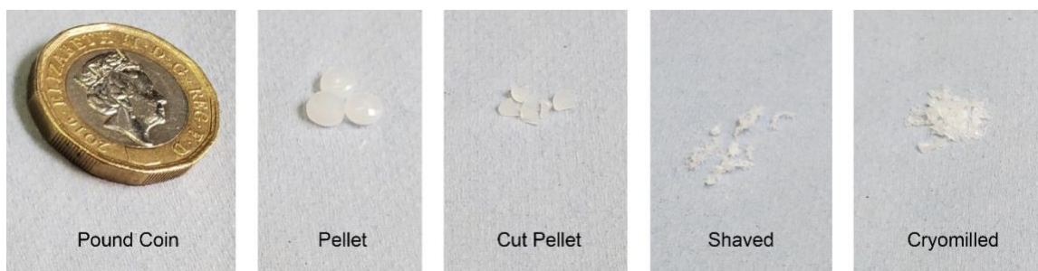
Figure 1. Comparison of the size and shape of the different forms of HDPE; commercial pellet with the three formulated samples (cut pellet, shaved and cryomilled) and a £1 coin for scale.
