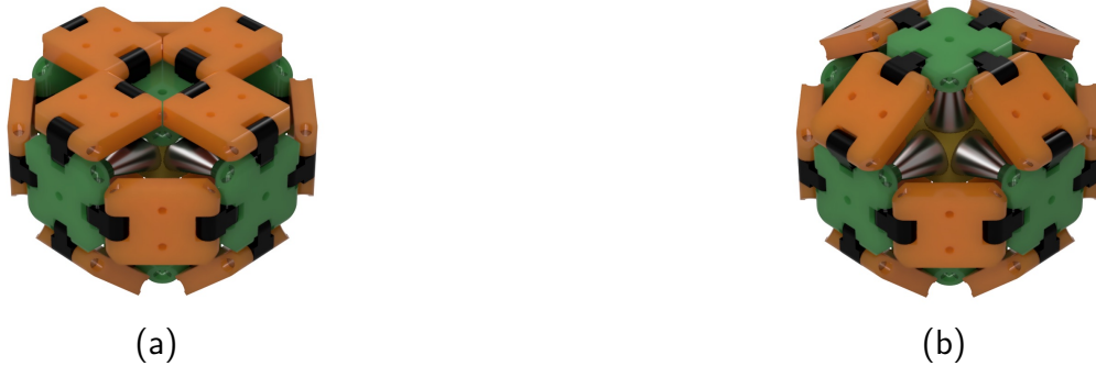
Figure 2: Representation of the two possible modes in which datoms can deform. A) Active deformation where the actuator is fully retracted and pull the A-face into the core causing the surrounding C-faces to lie on the same plane. B) Passive deformation caused by an external force which will cause a movement of the dome until the limits of the joints are reached.
