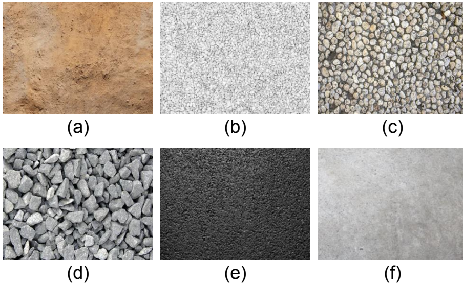
Figure 1: Images of various types of roads based on the materials used for road surfacing: (a) Earthen road, (b) Gravel road, (c) Kankar road, (d) WBM road, (e) Asphalt road, and (f) Concrete road.
