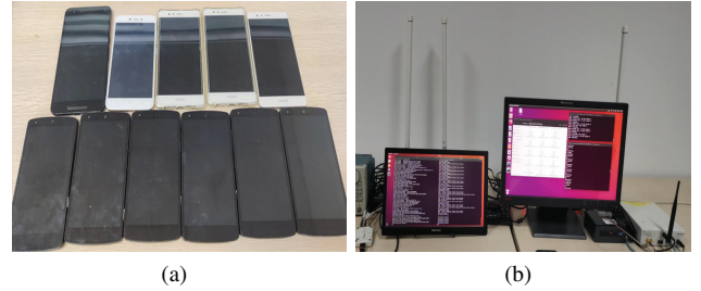
Fig. 11. (a) Photo of the ten LTE mobile phones. (b) Photo of the pseudo-LTE eNodeB station and the USRP receiver.
