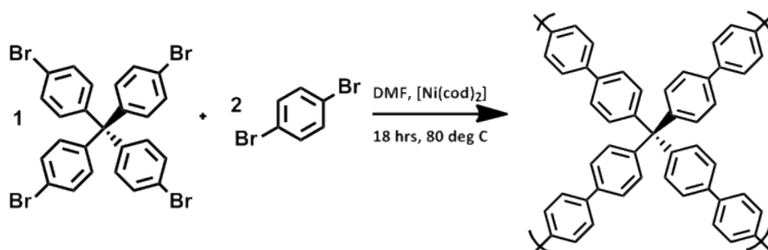
Figure 34: reaction scheme for the reaction between tetrakis(4-bromophenyl) methane and 1,4-dibromobenzene
