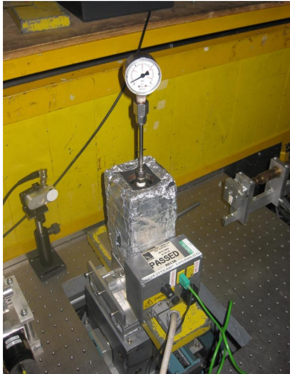
Figure 4 Apparatus set-up before measurements commenced, including the hydrothermal autoclave positioned within the thermal heating block.
