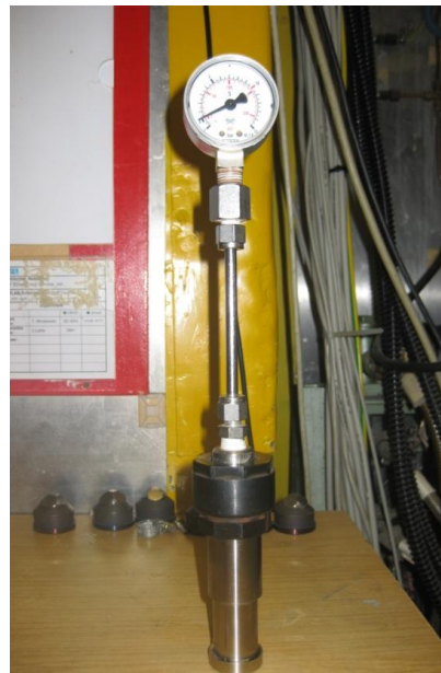
Figure 5 Adapted hydrothermal autoclave used for in-situ measurements.
