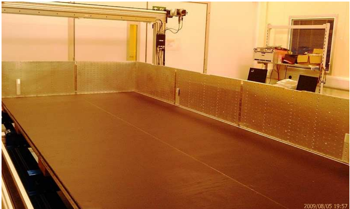
Figure 3.4: An assembled module base and bulkhead.
