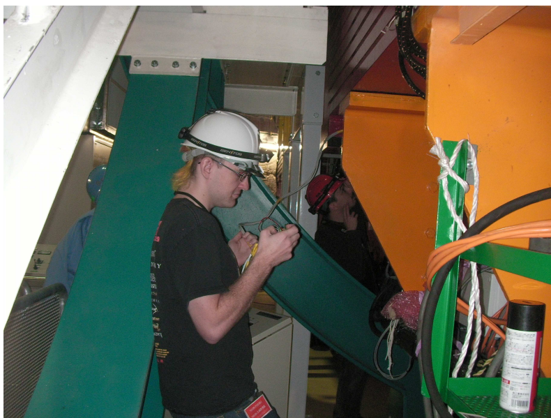
Figure 4.9: Monitoring the ECal touch strip sensors during magnet closure.
