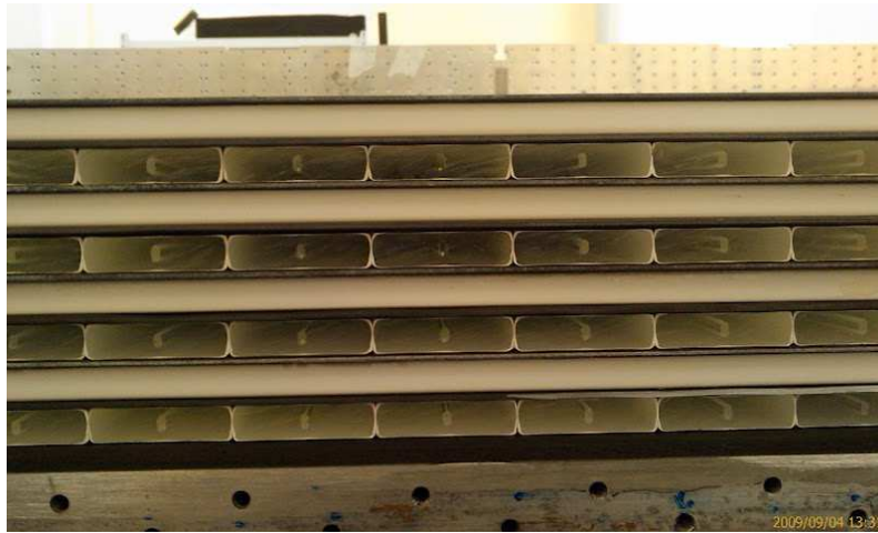
Figure 3.6: An end view of several ECal layers showing the lead-scintillator sandwich structure and the alternating orientation of the scintillator bars.
