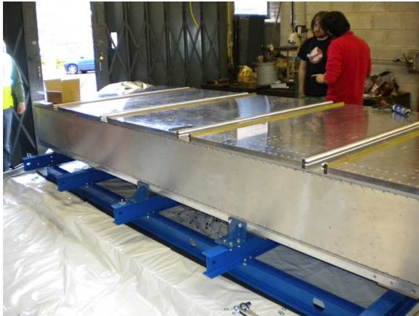
Figure 3.10: A completed barrel bottom ECal module. The grooves on top of the module are for sliding the module onto the metal beam that will eventually attach it to the ND280 magnet.
