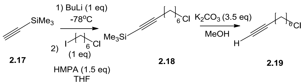
Scheme 2.9 Attempt to synthesise alkyne 2.19 via deprotonation of TMS-acetylene with BuLi and trapping out of the resulting lithio-species with chloriodohexane to give alkyne 2.18 , which was subsequently deprotected with K 2 CO 3 /MeOH.
