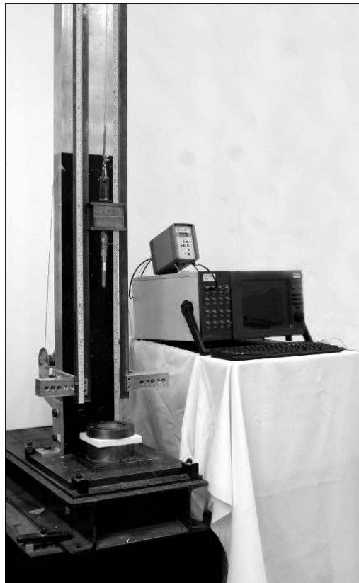
Figure 3.11 The low velocity impact tower.
