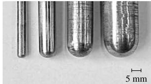
Figure 3.7 Photo of the hemispherical indentors used during the indentation test.
