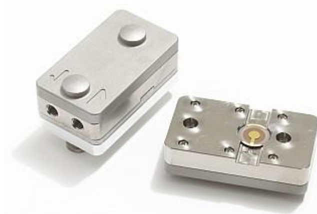
Figure 2.9: Q-Sense flow module with gold coated quartz sensor crystal in position. (Reproduced from www.q-sense.com ).
