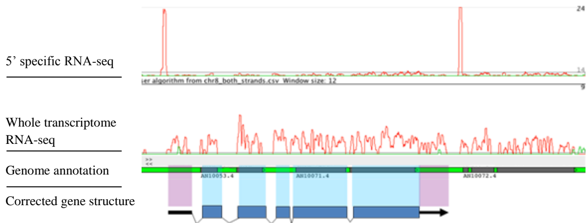
Figure 4.6. Correction of mis-annotation. Mapped RNA-seq coverage for the forward (green graph) and reverse (red graph) strands are displayed in Artemis against the forward (green track) strand of the A.nidulans genome assembly and the annotated exons in this region (dark grey). In this annotation (AN.4), two genes (AN10053.4 and AN10071.4) are predicted in this region. Whole transcriptome RNA-seq (lower graph) revealed the general structure of transcripts produced in this region. However, the uneven nature of the mapping makes accurate identification of the 5' end difficult. 5' specific sequencing (top track) gives a far clearer representation of the 5' end. Re-annotation of this region using the combined whole transcriptome and 5' RNA-seq data reveals that AN10053.4 and AN10071.4 lie within a single gene (bottom track) starting significantly upstream of previous estimates, including both previously annotated exons from both annotated genes (highlighted in blue), and two additional exons which had not previously been annotated (highlighted in pink). All RNA-seq data was produced from RNA extracted from A. nidulans culture grown on minimal media with nitrate (as previously described).
