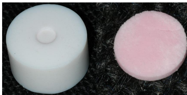
Figure (2): Mould used to make veneers with a porcelain veneer before firing.
