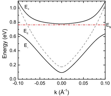
FIG. 2. (Color online) (a) Conduction band dispersion of  $\text{InN}_{0.01}\text{Sb}_{0.99}$  close to the  $\Gamma$  point of the Brillouin zone calculated using the  $\mathbf{k}\cdot\mathbf{P}$  BAC model. The host conduction band (dashed line) interacts with the N level (dash-dot line) and results in two conduction subbands  $E_-$  and  $E_+$  (solid lines).
