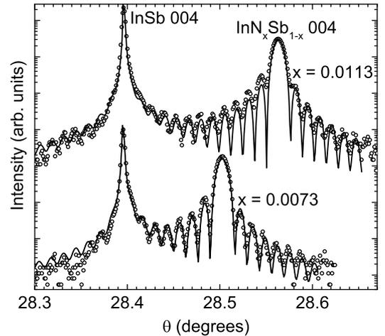
FIG. 1. XRD (points) of the 004 diffraction maximum from a InNSb films grown on a InSb substrate at  $275^\circ\text{C}$  at growth rates of 0.5 and  $1.75 \mu\text{m h}^{-1}$ . The results of the simulations (solid line) indicates that the InNSb films contain 1.13 and 0.73% N and their thickness are  $390 \pm 10$  nm and  $400 \pm 10$  nm, respectively.
