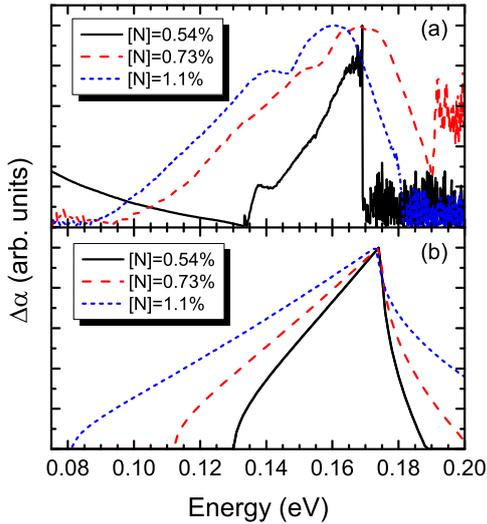
FIG. 3. (Color online) (a) Absorption spectra from  $\text{InN}_x\text{Sb}_{1-x}$  with  $x=0.54\%$  (solid line),  $0.73\%$  (dash line) and  $1.1\%$  (dash-dot line) grown on InSb substrates.  $\Delta\alpha$  denotes the difference in absorption by the InNSb film on InSb substrate and by InSb substrate alone; (b) The calculated absorption spectra within the BAC model.
