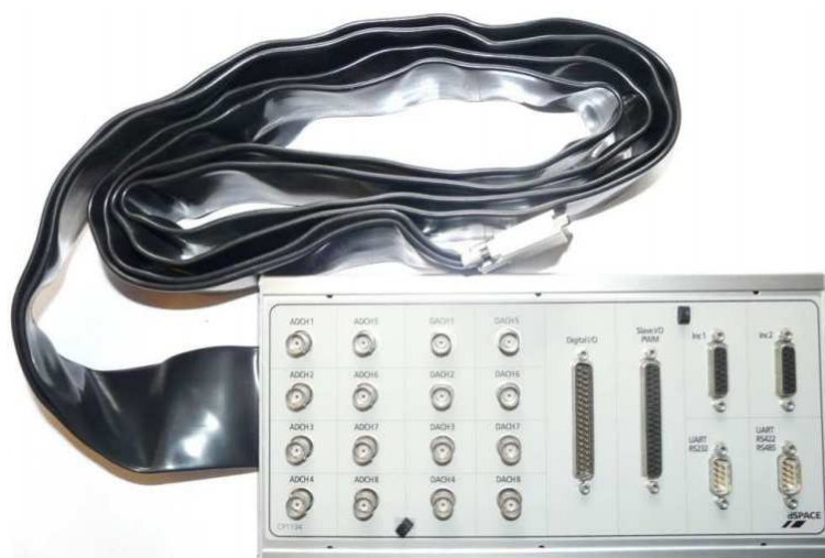
Figure 6.12: The DS1104 control panel of dSPACE with ADC/DAC interface.
