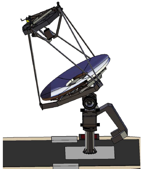
Figure 1: Computer model (using the CATIA software) of the SST-GATE telescope. The camera is located between the primary and secondary mirror.
