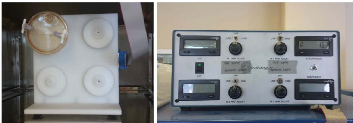
Figure 4.2.1 Rotary cell culture system (RCCS) setup. The annotated image shows a typical RCCS setup using a 50 mL disposable culture vessels. The RCCS culture system (left) would be placed inside the incubator, with the control box (right) placed outside and linked via cable.
