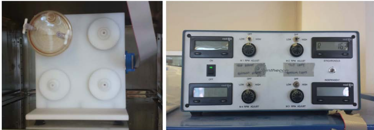
Figure 8.4. Rotary cell culture system (RCCS). The annotated image shows a typical RCCS setup using a 50 mL disposable culture vessel. The RCCS culture system (left) would be placed inside the incubator, with the control box (right) placed outside and linked via cable.
