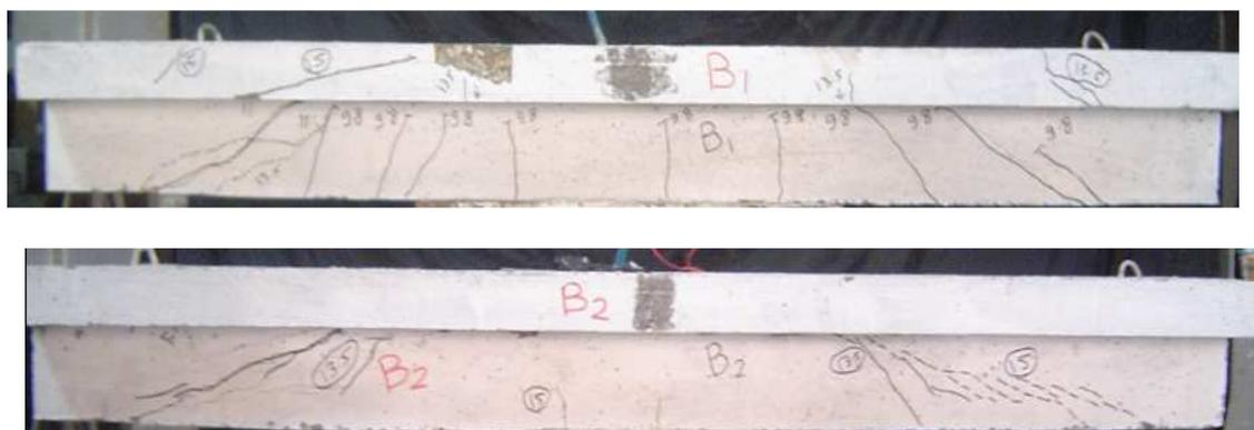
Fig.2: Cracking pattern for beams B1 and B2
