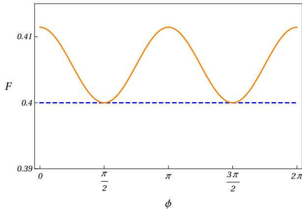
**Figure 4.** Modulation of the response function  $F$  of eq (3.26) as the interferometer rotates an angle  $\phi$  around an axis aligned with one of the interferometer arms. We assume that this arm points along the earth’s rotation axis, and we choose a reference frame so that it corresponds to the direction  $\hat{x}$ . The dashed blue line shows the case with no anisotropy,  $Q_{ij} = 0$ , whereas the orange line shows the case with one component  $Q_{33} = -Q_{11} = 0.1$  turned on.
