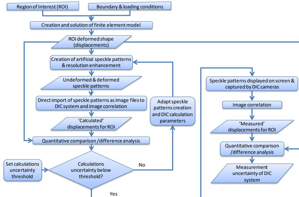
**Fig. 1.** Methodology of DIC uncertainty quantification based on un-deformed and deformed speckle patterns.
