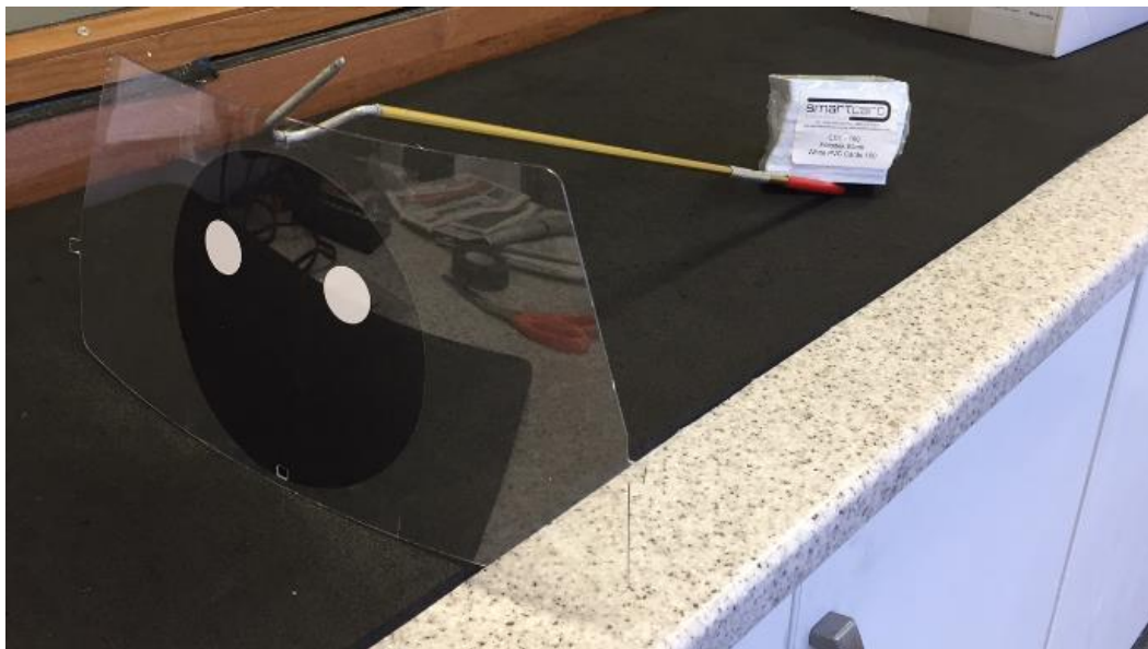
Fig. 6.2. The setup for collecting spat venom. This utilises an isolated mask visor, snake hook and printed paper bearing the “face” design depicted in Fig. 6.1.
