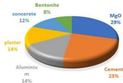
Figure 3: Figure 1: Most contributing materials (Global Warming) in MgOSIP house.
