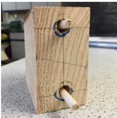
Figure 2: Two micro clear specimens cored from a block cut from a structural sized joist (specimen 'A' top, and 'B' bottom)
