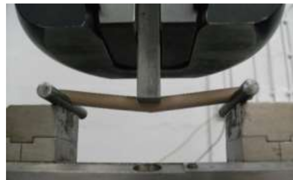
Figure 5: Three point bending of a micro clear specimen just after failure has occurred
