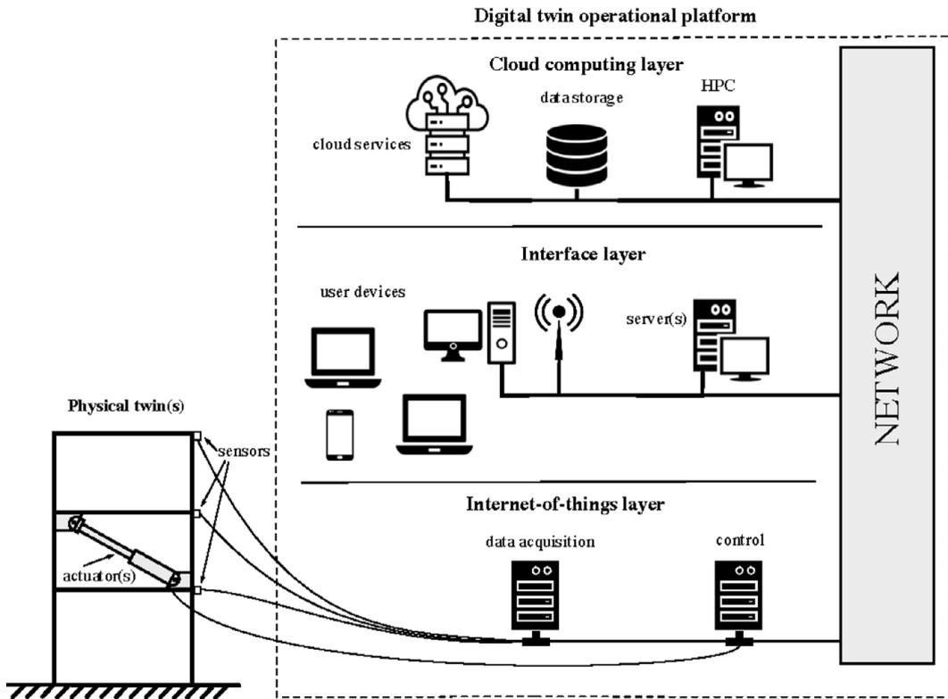
**Figure 2.** A schematic representation showing the three “layers” of a browser-based digital twin operational platform (DTOP). Note that (a) the sensors and the actuators are part of the IoT layer, but shown here outside the DTOP dashed box for convenience, and (b) the actuator system shown in the IoT layer is for conceptual insight only, and it is not supposed to represent a typical actuator configuration in a three-storey structure.
