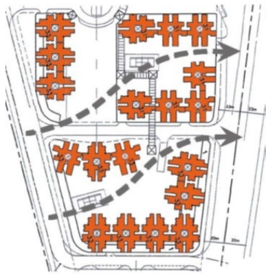
1. Site disposition to provide air paths
