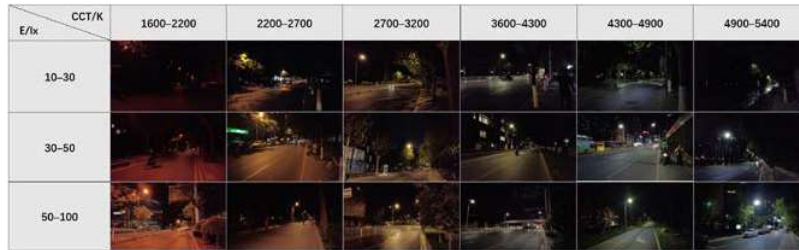
Figure 2. Images of roads with different color temperature and illuminance combinations
