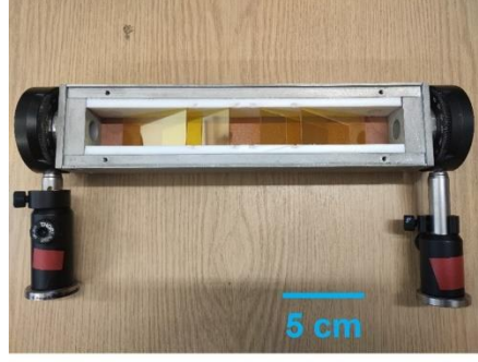
Fig. 2. Photo of the 4 plate POP polariser device using rectangular polycrystalline ZnSe plates, 1.0 mm thick with separation 26 mm along the optic axis, avoiding multiple reflections between plates. The assembly was supported on rotational stages either end.
