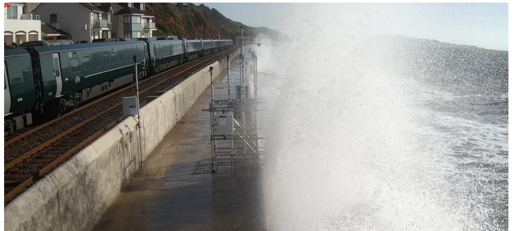
Figure 3: A hard-engineered coastline with railway infrastructure and a new wave overtopping measurement system, 'WireWall'. Photo from the University of Plymouth's Dawlish camera installed as part of the Coastal REsistance: Alerts and Monitoring Technologies (CreamT) project.
