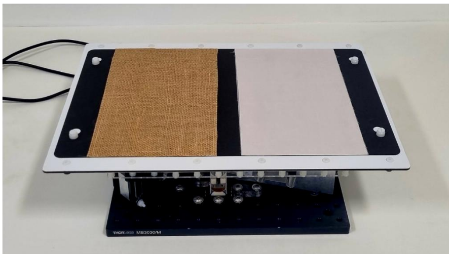
Figure 6.3 Set up of the six axis sensor with the load cells connected to the junction boxes (A), and with the ACP fitted (B). Textures mounted the the paper sample mount and fixed to the ACP (C).
