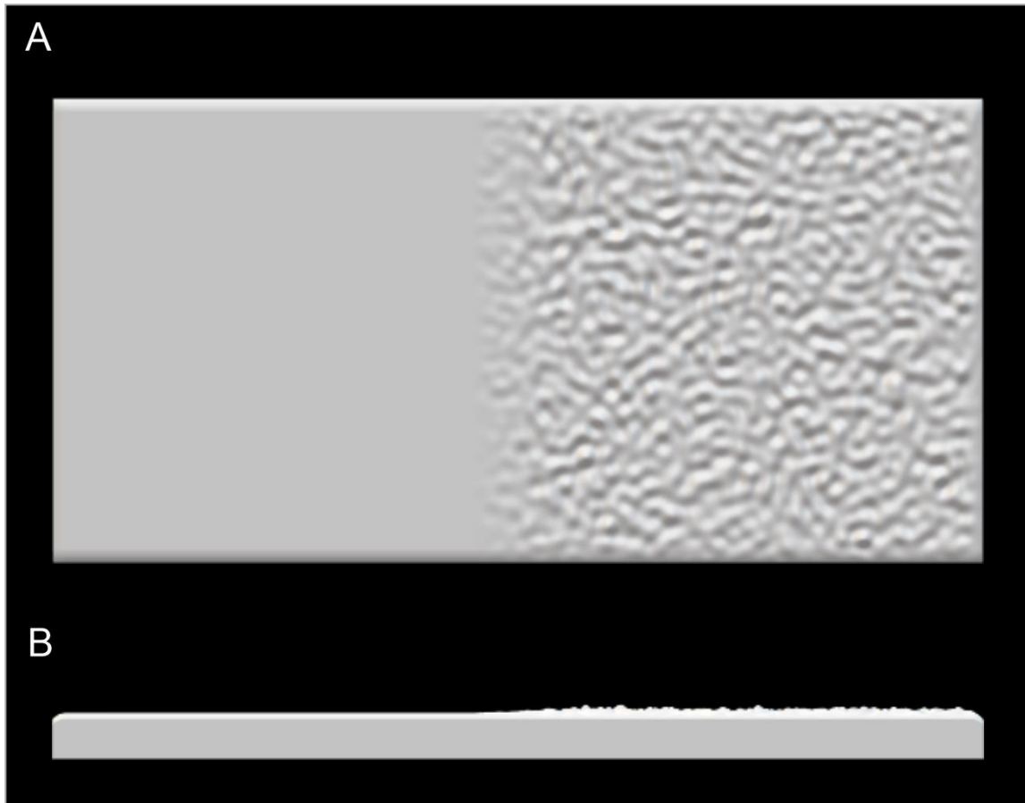
Figure 7.1 3D printed stimuli 100 mm × 50 mm where left is the smooth portion of the tile and right is the rough portion of the tile. Superior (A) and horizontal view (B).
