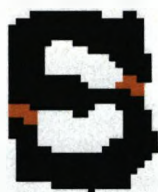
Figure 5.35: A character with its uncertain areas set in orange. The number of uncertain areas is 2; the number of possible characters is 2^2 = 4 .
