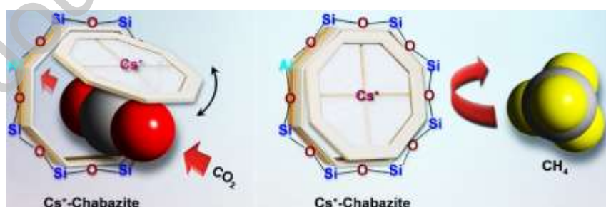
Figure 3.38. Illustration of the “molecular trapdoor” mechanism in discriminative gas separation: Cs + locating in the middle of 8MR acts as a doorkeeping cation, which can only be deviated by strong gas molecules (e.g., CO 2 ), but not by weak molecules (e.g., CH 4 ) at certain temperature. (Shang et al., 2012)
