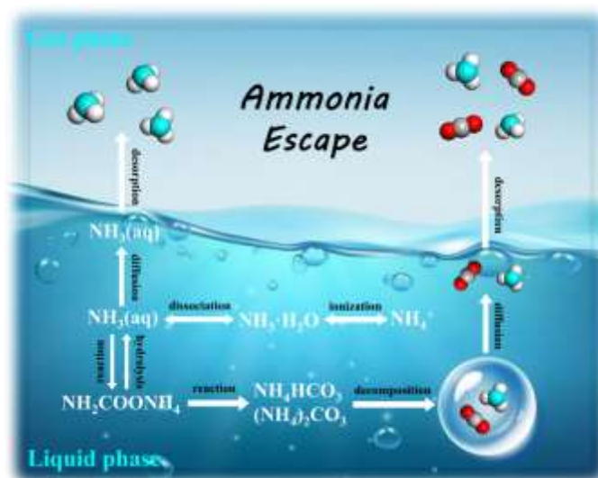
Figure 3.2 Schematic diagram of ammonia escape.
