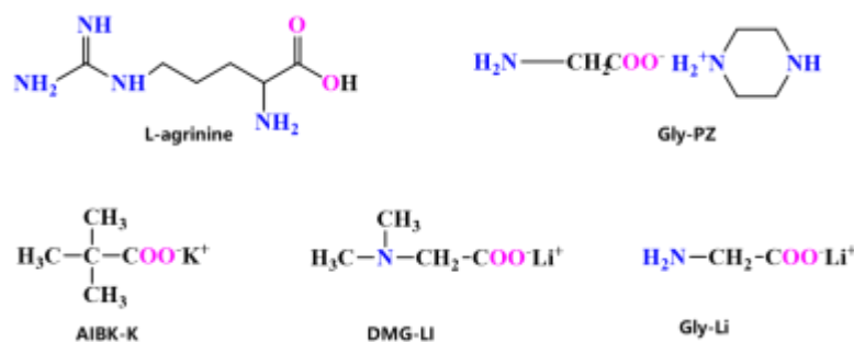
Figure 4.12. Typical mobile carrier used in FT membranes, reproduced from (Zhang, Z. et al., 2021)
