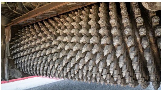
Fig. 75. Fine milling rotor with 672 cutters.
