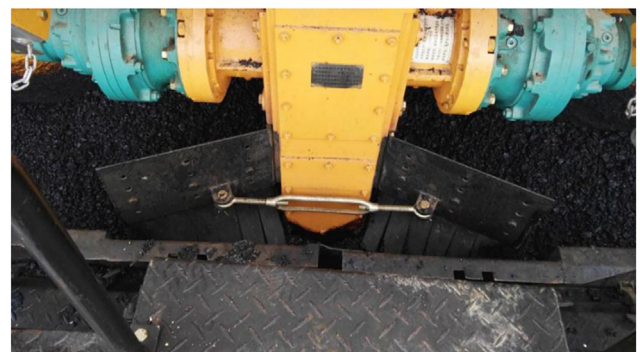
Fig. 72. Installation of rubber baffle in screw gearbox.
